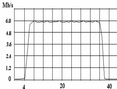
**Figure 6** Network throughput for the wired point-to-multipoint link
