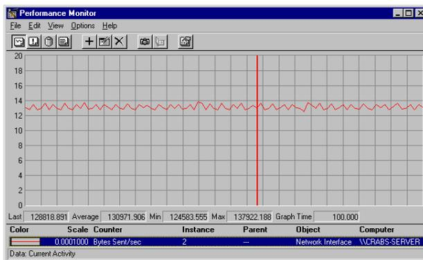
*Figure 8 Actual transmission rate (of an MPEG-1 file with stream bit-rate at 1Mbps) Versus Time*
