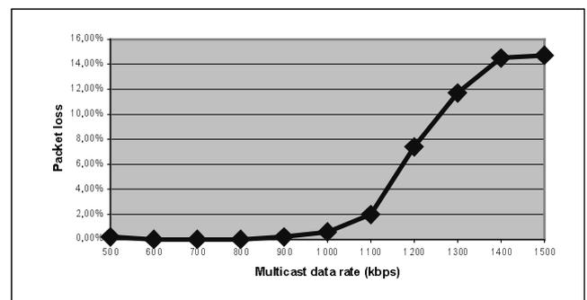
**Fig. 5 Data packet loss vs. multicast rate**
