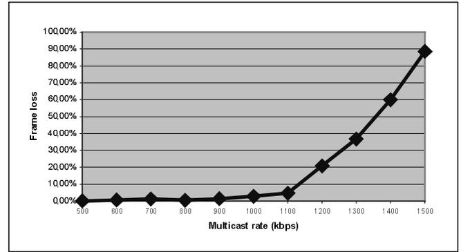
**Fig. 7 Video frame loss vs. Multicast rate**
