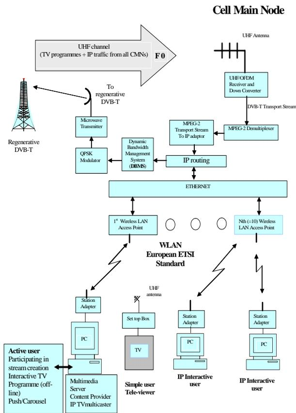
**Fig. 4 Overall configuration of the CMN with WLAN**
