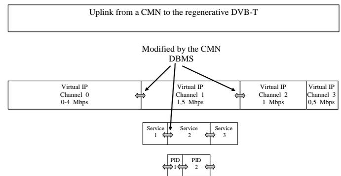
**Fig. 5 Bandwidth slicing in a DVB-T transport stream**
