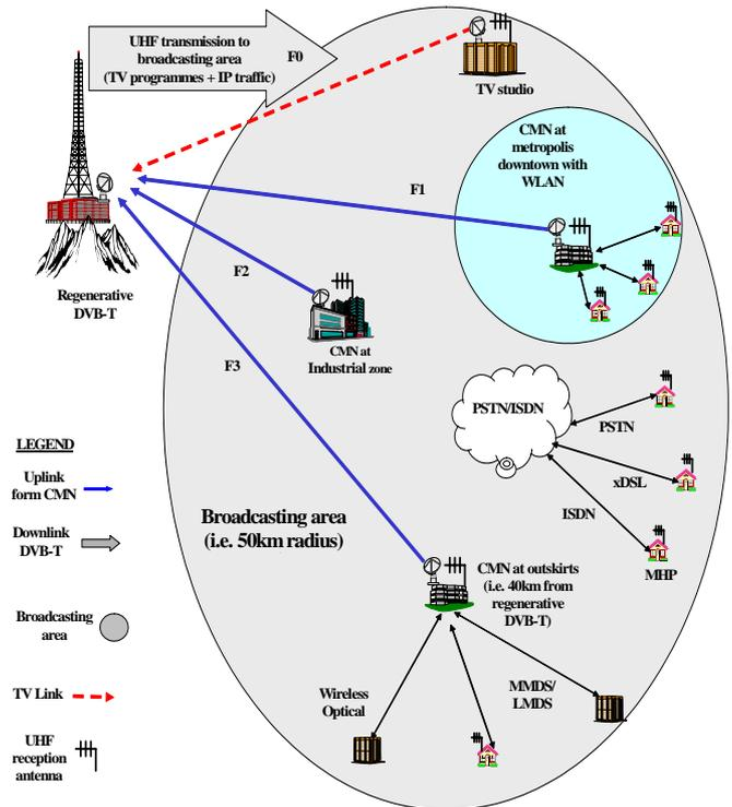
**Fig. 1 Overview of the network configuration, where the common Ethernet backbone, access by both active and passive users/citizens, is present in the entire broadcasting area**
