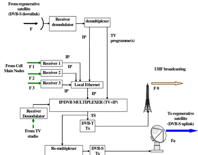
Fig. 3 Overall configuration of the regenerative DVB-T
