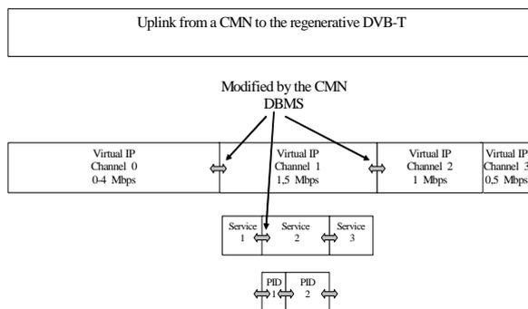
Figure 5. Bandwidth slicing in a DVB-T transport stream.
