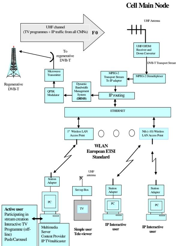
Figure 4. Overall configuration of the CMN with WLAN
