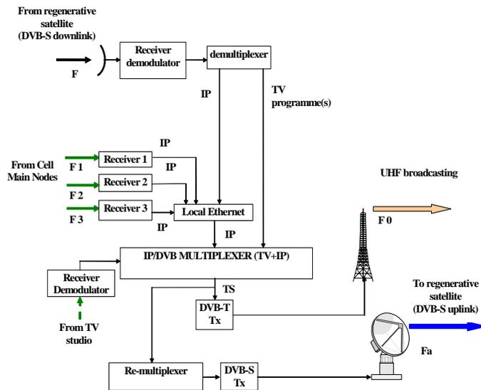
Figure 3. Overall configuration of the regenerative DVB-T
