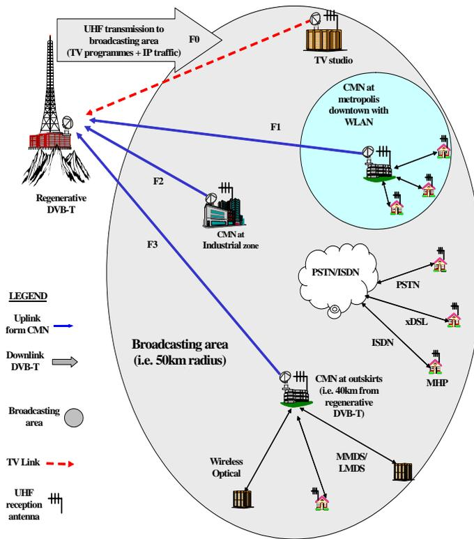
Figure 1. Overview of the network configuration, where the common Ethernet backbone, access by both active and passive users/citizens, is present in the entire broadcasting area
