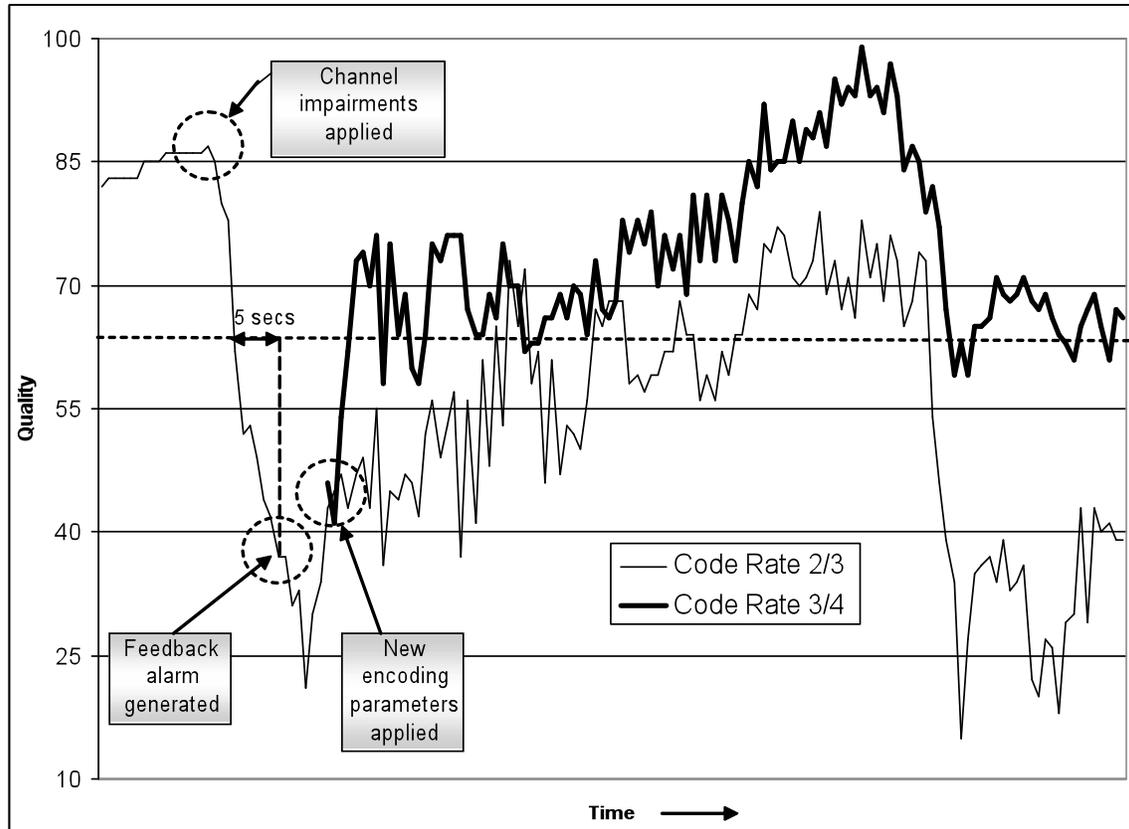
**Figure 3.** PQoS Measurements over fading and noisy DVB-T channel, with and without feedback implementation.
