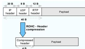
Figure 1: Robust header compression operation.
