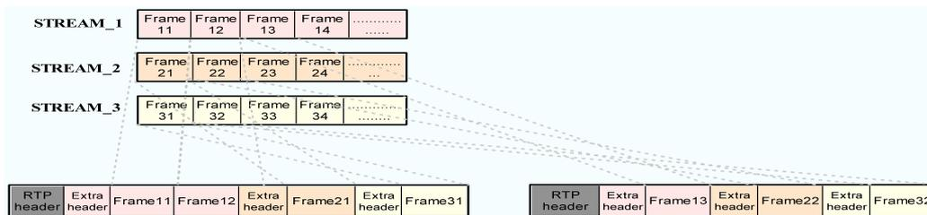
Figure 2: Multi-level RTP packet multiplexing and aggregation protocol.
