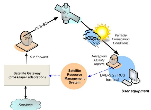
Figure 1. General concept of the SRMS closed-loop control system
