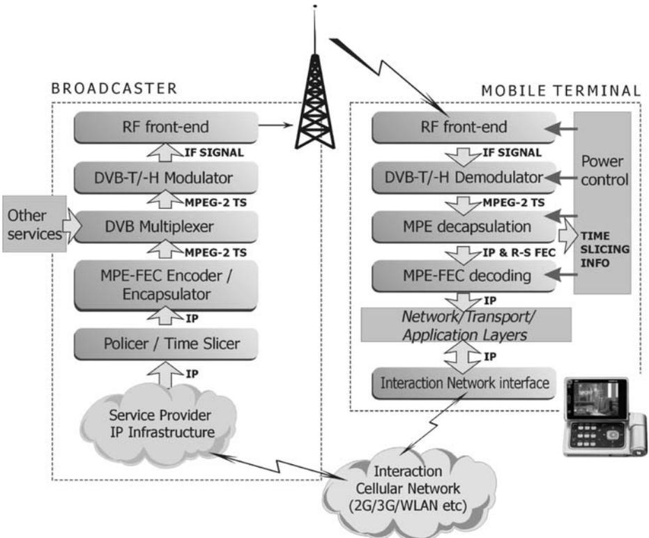
Fig. 1 Block diagram of a DVB-H system
